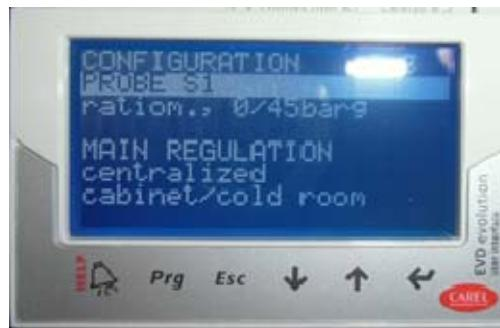
9. With "Arrows down" go to the next steps and check all connections as shown on display
