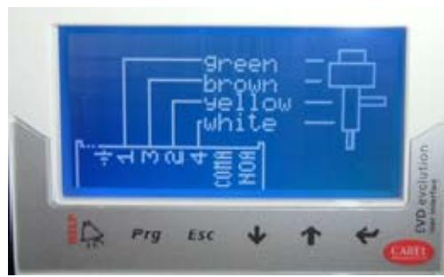
10. Once on **END CONFIGURATION** display, move with "Arrows up-down" to **YES** and push ↵
